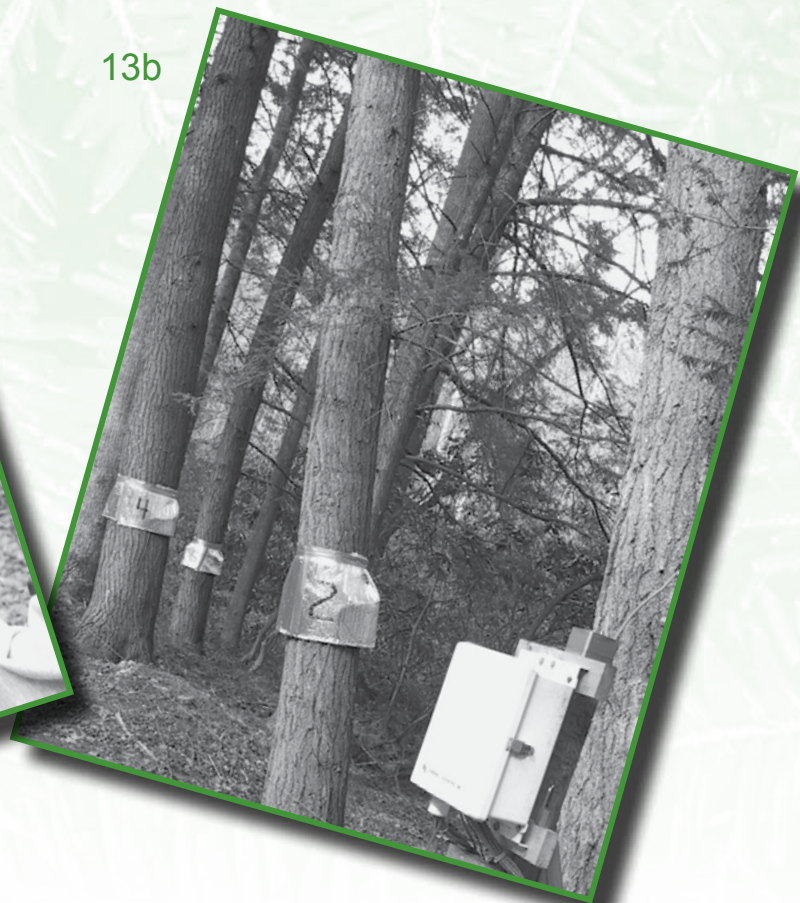
Figures 13a and 13b. The probes were placed into the tree's sapwood.
